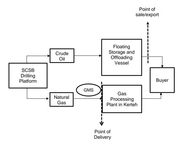
Based on this example, point of sale or export for crude oil is at floating storage and offloading vessel while the point of delivery for natural gas is at GMS delivery point of the Gas Processing Plant in Kerteh.
